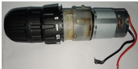
Fig.2. D.C. Geared Motor (12V)
