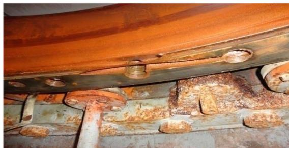
**Fig:2 Eroded Bottom Ring**
